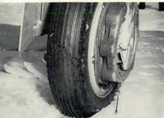
Tire damage caused by locking wheel during braking run on slush.
