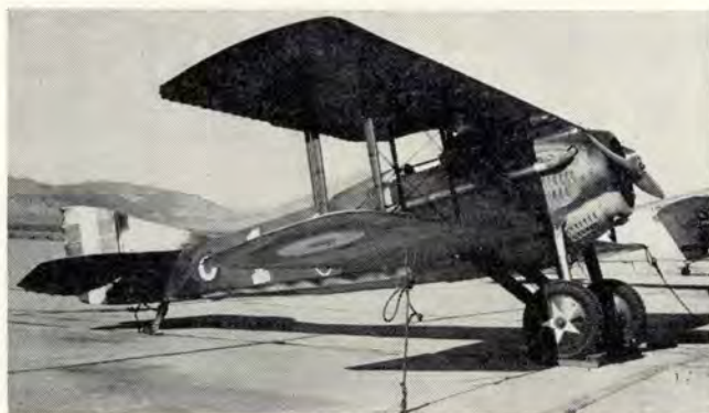
An early vintage fighter sports a fixed pitch wood propeller; simple, but most inefficient by today's standards.
