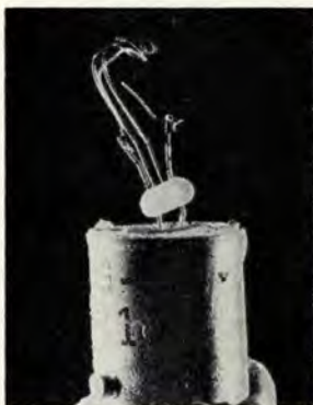
Left, typical case of a small filament shocked in the heated state. Right, small filament shocked in cold state.
